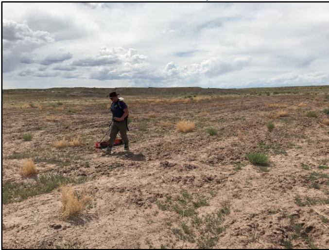
Scanning of a field site with a hand-held EMI device.
